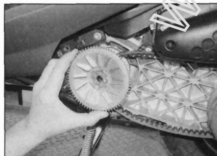
4.22a Install the outer pulley half . . .
