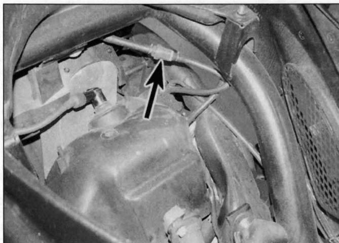
11.4 Inspect the oil filter (arrowed)
