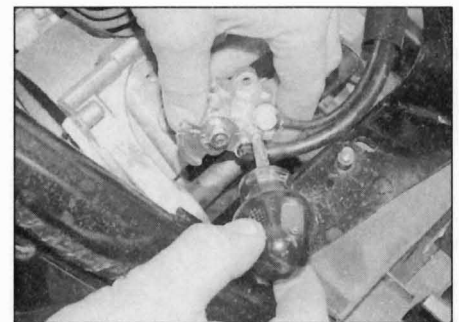
13.19b Bleeding a cable operated oil pump
