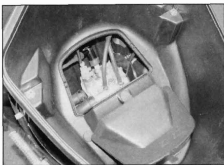
17.1a Open the engine access panel . . .
