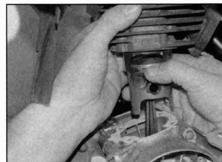
8.2 Support the piston as the cylinder is lifted off
