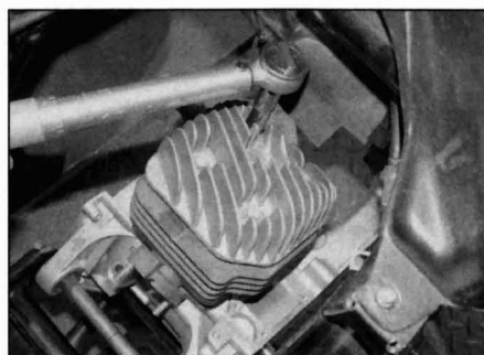
7.3 Unscrew the cylinder head bolts evenly in a criss-cross sequence
