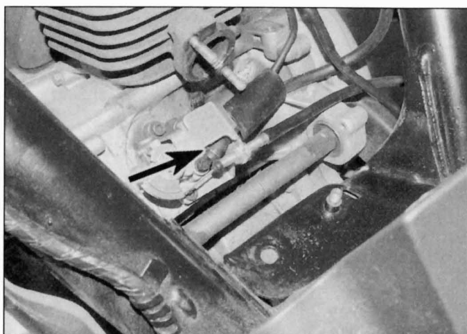
11.5a Inspect oil hose connections (arrowed) for possible leaks
