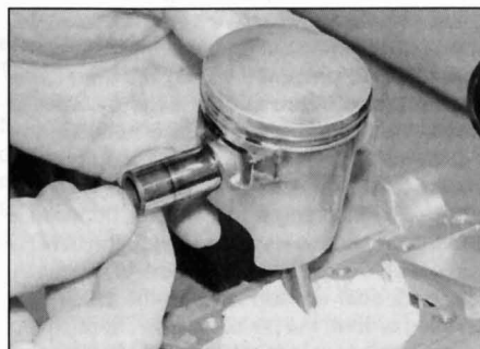
9.3b ... then push out the piston pin
