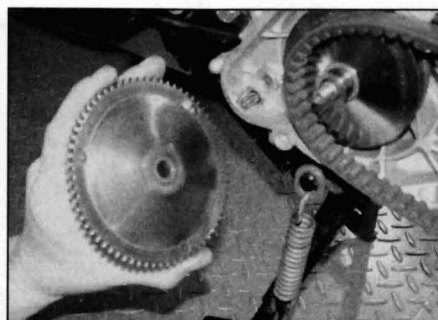
4.3b . . . then remove the outer half of the pulley
