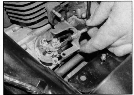
5.10 Remove the oil pump cable and bracket
