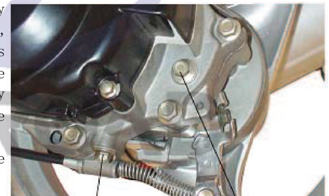
Draining bolt of gear oil
