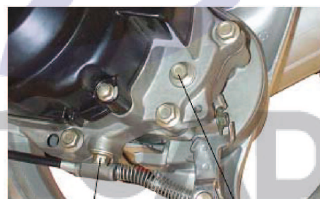
Draining bolt of gear oil
