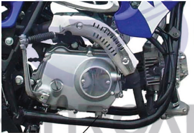
screw plug for oil draining
