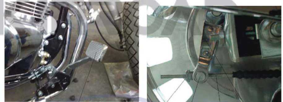
Adjusting nut Brake arm pin Rear brake arm Brake pull rod
