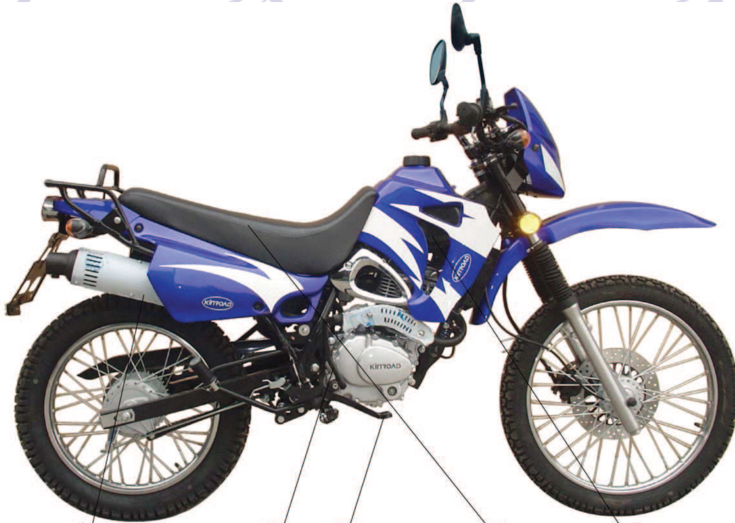
1. exhaust silencer 2. kick lever 3. rear braking pedal 4. seat cushion 5. fuel tank
