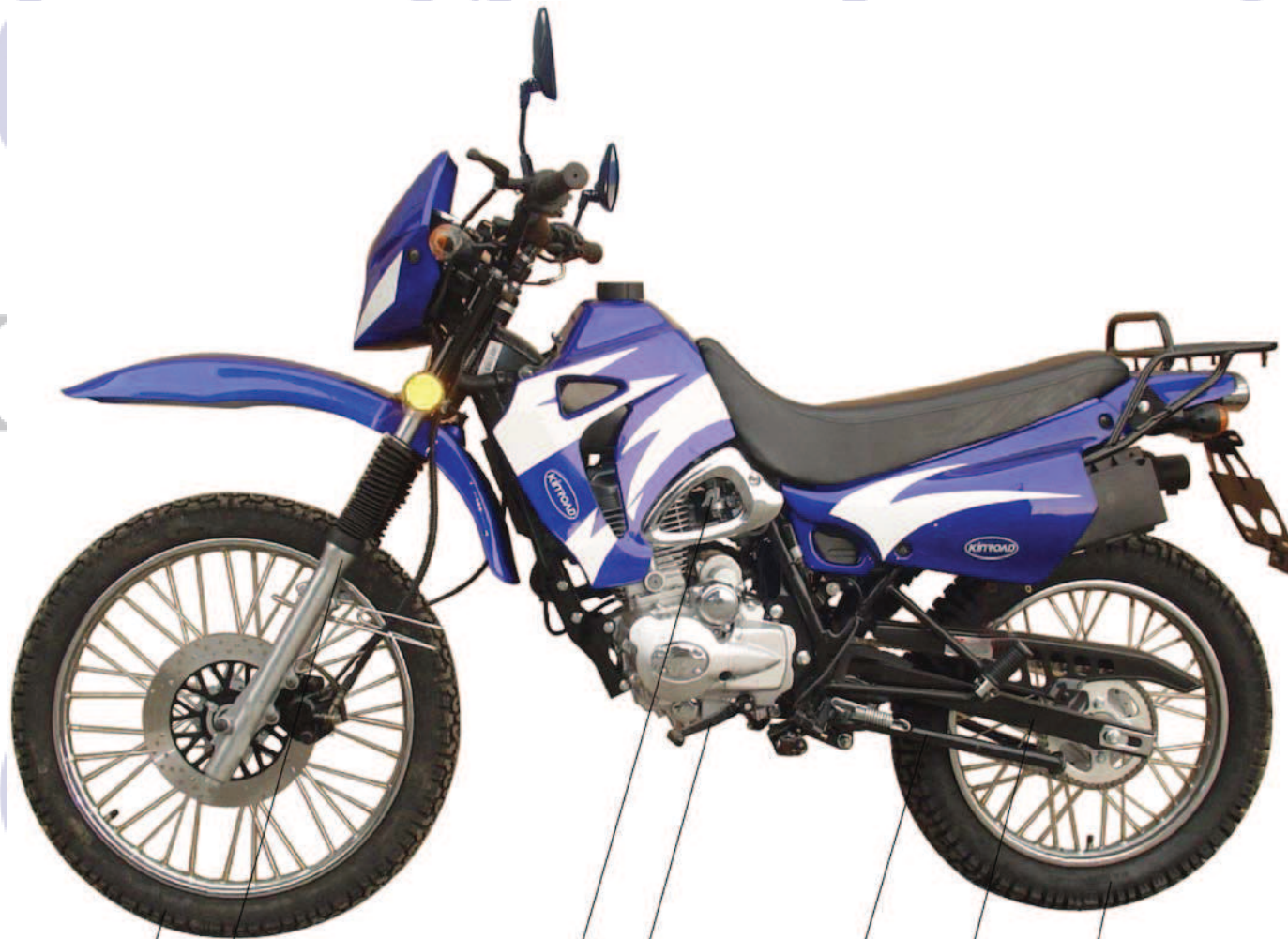
1. front wheel 2. front shock sbsorb 3. fuel cock 4. gear shifting 5. side stand 6. rear fork 7. rear wheel
