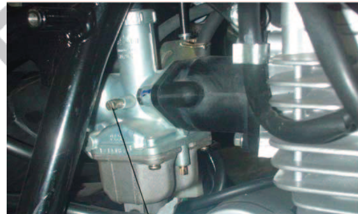
Idling speed adjusting screw
